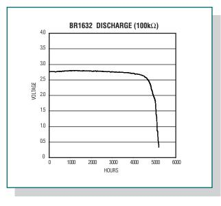
Figure 2. The output voltage remains constant during discharge.
