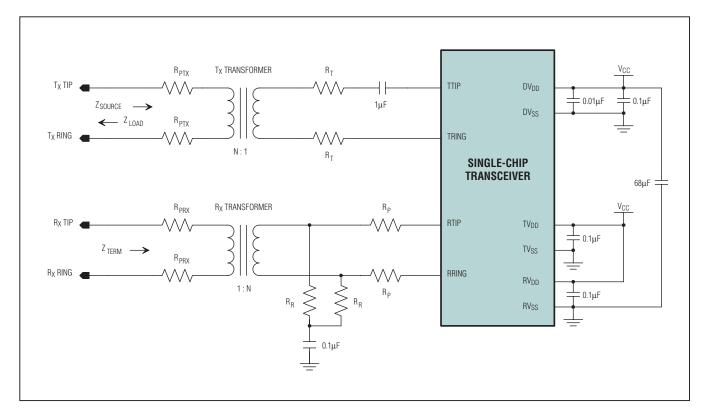
This traditional interface circuit for T1/E1 devices illustrates how resistance is distributed around transformers. Using the model as the baseline circuit for network interface design, users can better understand secondary voltage protection for the DS2155. (See article inside, page 3.)
