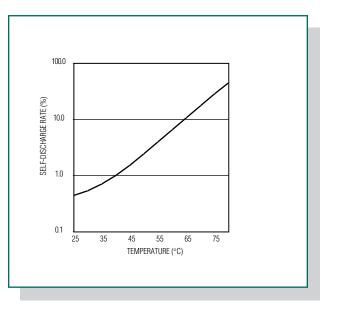
Figure 4. The self-discharge rate increases as temperature increases.
