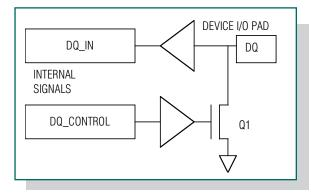
Figure 1. DQ pad driver (one\_wire\_io) must be an open-drain pad with the proper ESD protection.
