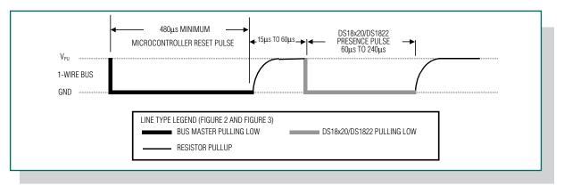
Figure 2. Every communication cycle begins with a reset pulse from the microcontroller followed by a presence pulse from the DS18x20/DS1822.
