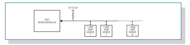
Figure 1. Multiple 1-Wire temperature sensors can be connected to a single-wire bus.
