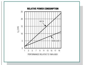
Figure 1. Reduced clock cycle core uses less current for same throughput.
