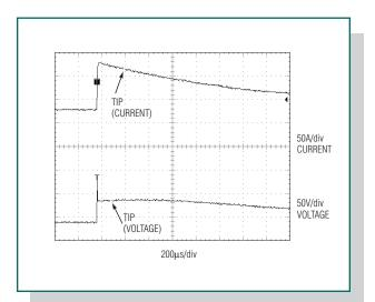
Figure 6. Initial surge clamping at tip input
